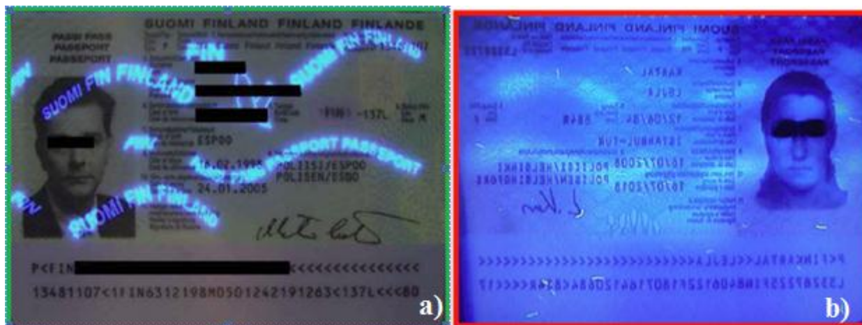
Fig. 9. Exposure under UV light of a genuine document (a) and of a forged (b)
